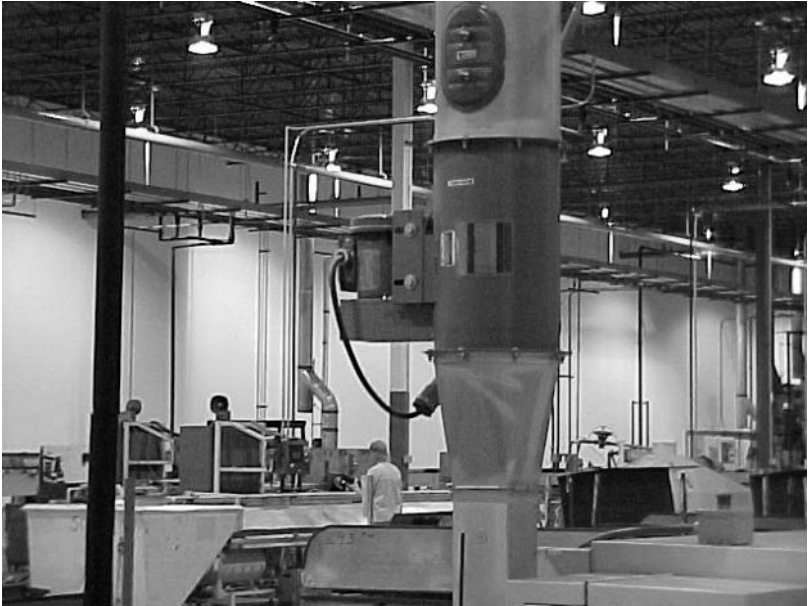
Figure 8-2. What would cause this 1 HP fan to have a high failure rate?
