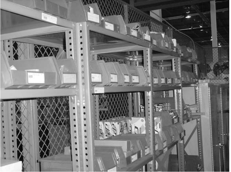
Figure 7-1. Plastic bins for storing spare parts.
