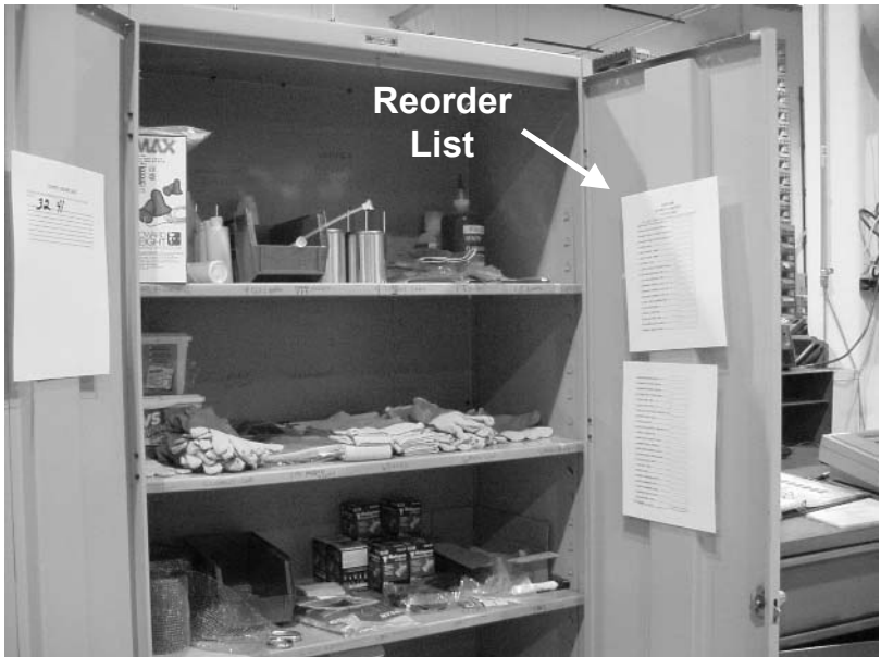
Figure 7-5. Expendables cabinet, with reorder list posted on the door, reduces the time spent searching for everyday supplies.
