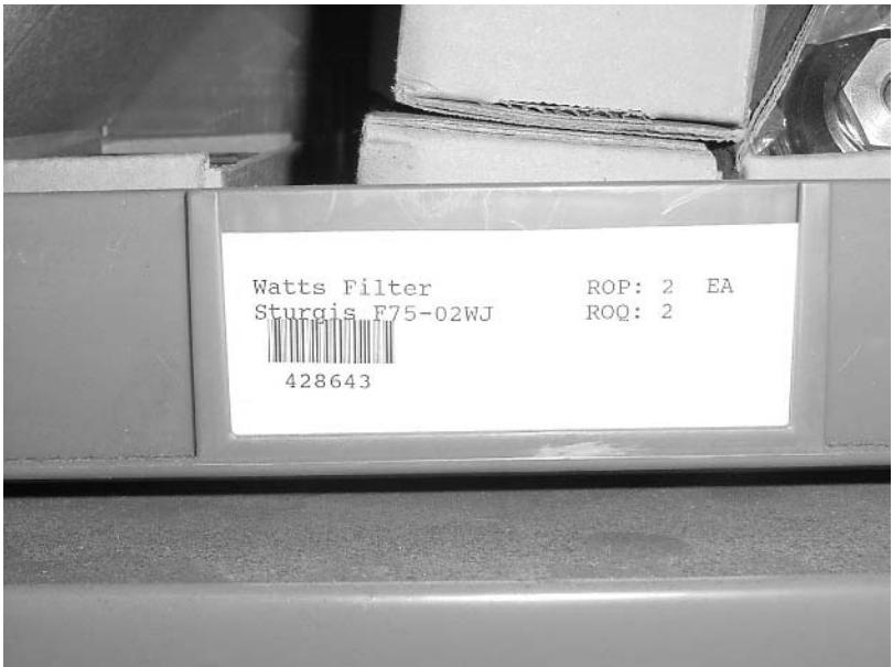
Figure 7-6. Adding barcodes to the bin labels allows implementation of an electronic ordering system.
